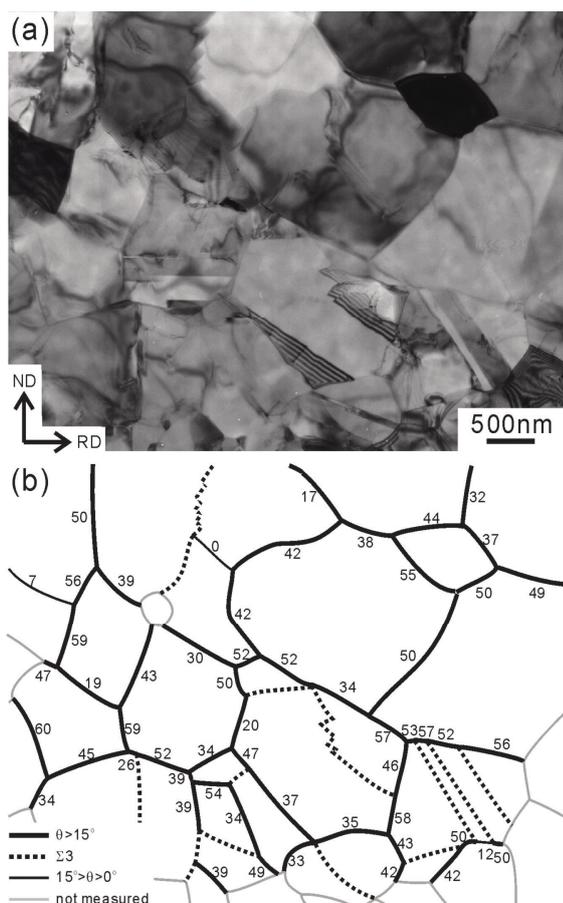
Fig.1 Bright field image (a) and corresponding misorientation map (b) of the TWIP steel 88% cold-rolling and annealed at 620°C for 1.8ks.
