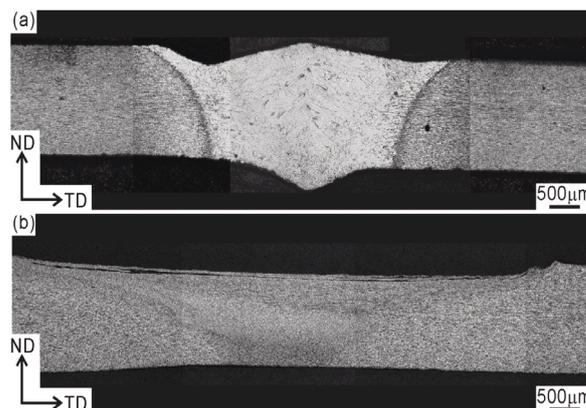
Fig. 2 Optical micrographs of the transverse sections of the welded zone in the TWIP steel. (a) TIG welding and (b) FS welding..
