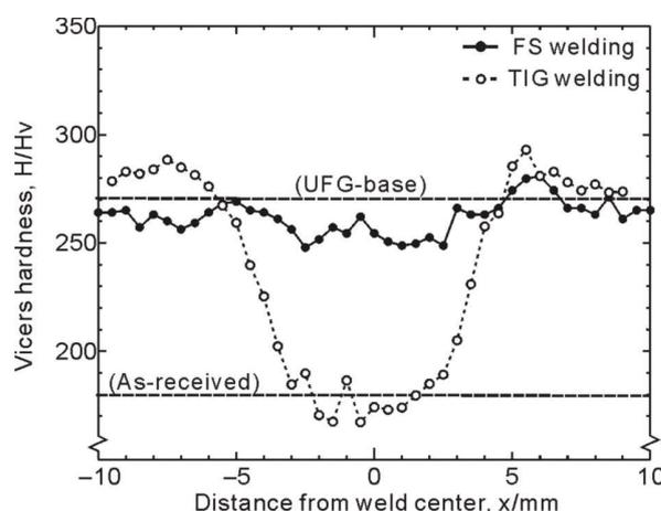
Fig. 3 Hardness profiles of FSW/TIG welded joints of TWIP steels 88% cold-rolled and annealed at 620°C for 1.8ks.
