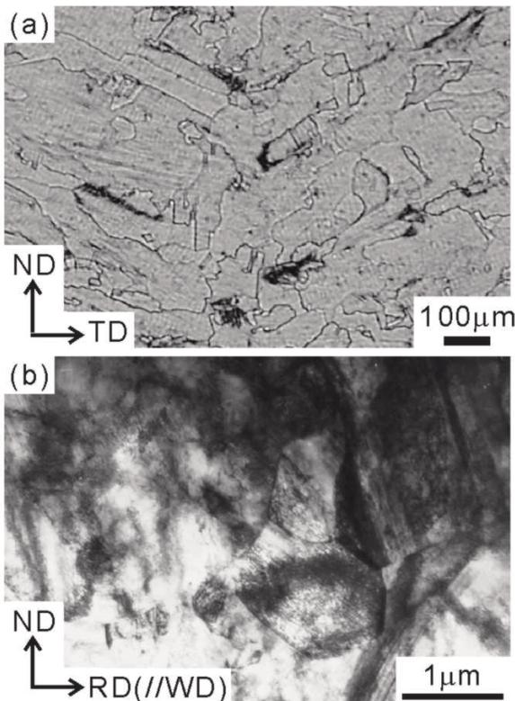
Fig. 4 Optical microstructure of the TIG welded joint (a) and TEM bright field image of the FS welded joint (b).
