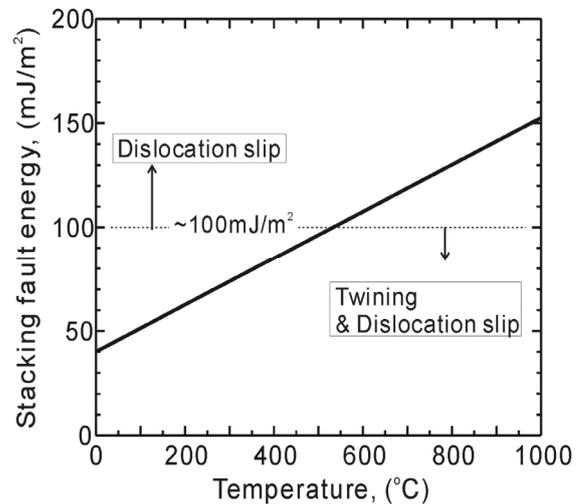
Fig. 5 Stacking fault energy of TWIP steel as a function of temperature.
