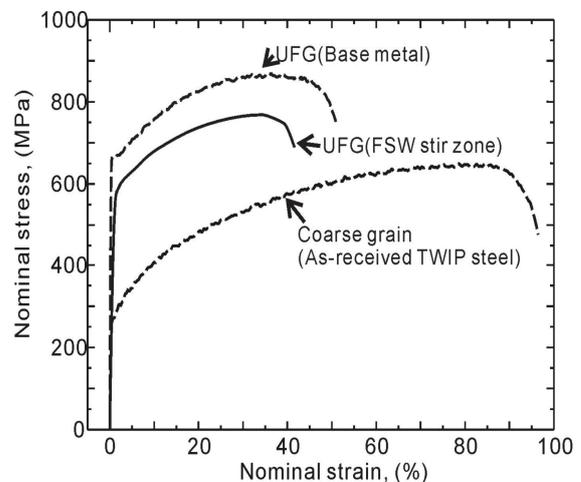
Fig. 6 Nominal stress – nominal strain curves of TWIP steels.
