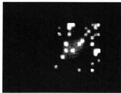
Fig. 6.12: Encoded and multiplexed bit planes after propagation through image fiber.
