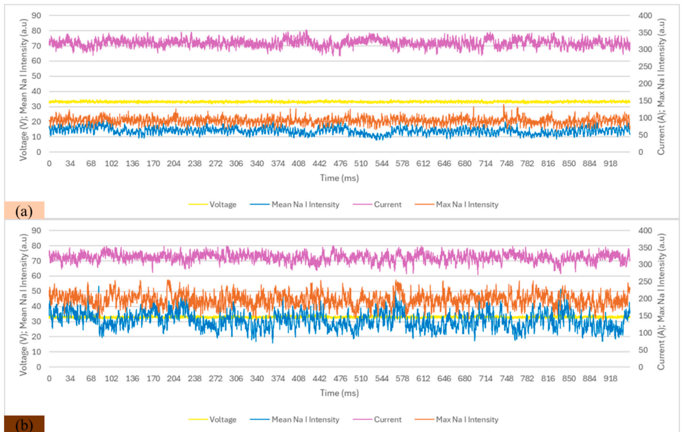
Fig. 22. Current, voltage and intensity waveform for (a) wire 1 and (b) wire 4 at welding current of 310 A.
