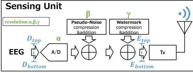
Fig. 2. Schematic of the transmitter.  $D_{top}$  and  $D_{bottom}$  represent the upper and lower limits of the signal range for the A/D converter, respectively. Similarly,  $E_{top}$  and  $E_{bottom}$  represent the upper and lower limits of the signal range for the transmitter.  $\alpha$  is the resolution of the A/D converter,  $\beta$  is the resolution of the pseudo-noise, and  $\gamma$  is the resolution of the watermark.
