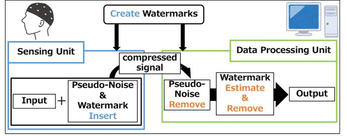
Fig. 1. In the proposed method, a watermark is created in advance, which is shared by the sensing and data processing units. The sensing side generates pseudo-noise using a seed value based on the watermark. The processing side receives a compressed EEG signal that is a combination of the EEG, watermark, and pseudo-noise. The pseudo-noise and watermark can be eliminated by using the pre-shared watermark information.
