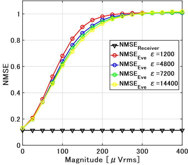
Fig. 5. This graph represents the average NMSE over 1000 frames when the proposed method and eavesdropper attempt to reconstruct brainwave signals with arbitrary pseudo-noise inserted. Here,  $\epsilon$  indicates the number of pairs of input signals and compressed signals obtained by the attacker.
