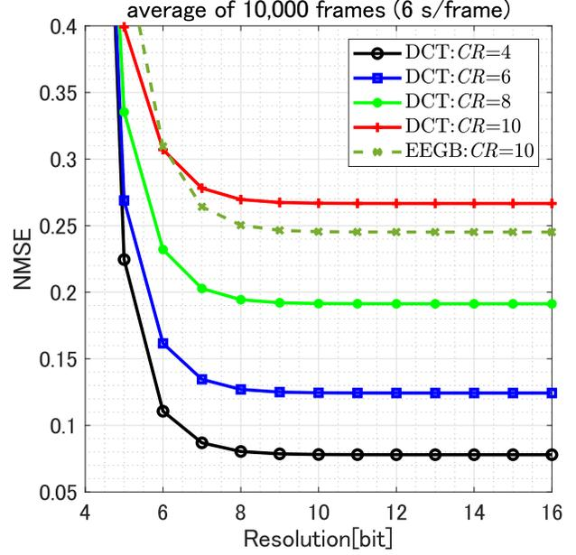
Fig. 6. This graph illustrates the resolution dependence of reconstruction accuracy for various compression ratios when adding a  $100 \mu\text{Vrms}$  watermark and  $250 \mu\text{Vrms}$  pseudo-noise to the EEG data. The solid line represents data using DCT, while the dashed line represents data using EEGB.
