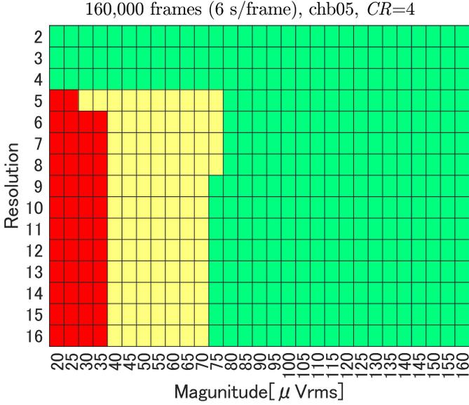
Fig. 3. Shmoo plot showing the magnitude of watermark and estimation accuracy for each resolution. The estimation accuracy is represented by different colors: the red area indicates less than 99.8 %; the yellow area indicates between 99.8 % and less than 100 %; and the green area indicates 100 %.
