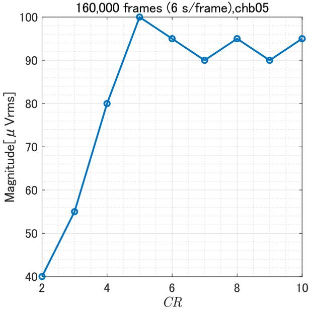
Fig. 4. This figure illustrates the magnitude of the watermark necessary for reliable watermark estimation for each CR.
