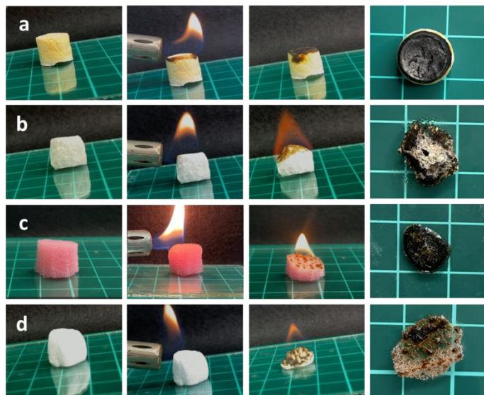
Figure 2-7. Photographs demonstrating the behavior under open flame of (a) CSNFs-DACMC (2.5 wt%, FT -25 °C, TT 4 °C), and commercial (b) cellulose, (c) PU, and (d) PS foams.
