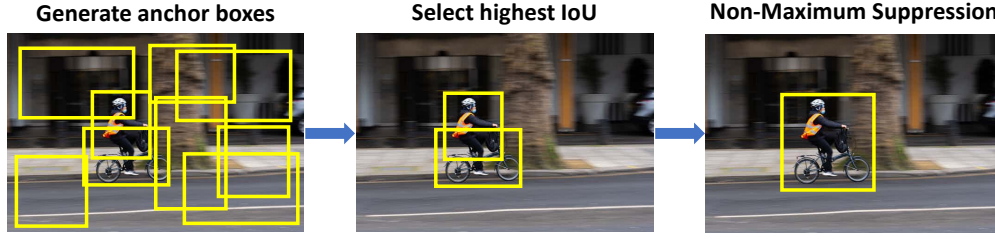
Figure 2.3: The object detection using R-CNN and Fast-RCNN.
