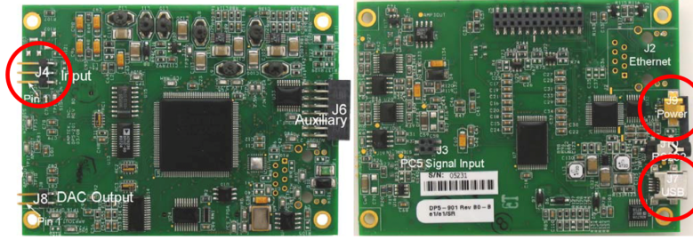
Figure 2.13: Front and back view of the DP5. Red circles indicate the main connections (input, power and communications)
