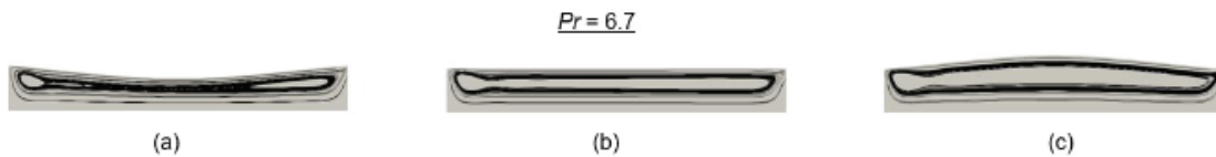
Figure 4.19 The streamlines for (a) S = 0.8 (b) S = 1 (c) S = 1.2 at the x - z plane along AB line ( y = 5 mm) at ( Ma_T = 5 \times 10^3 ).
