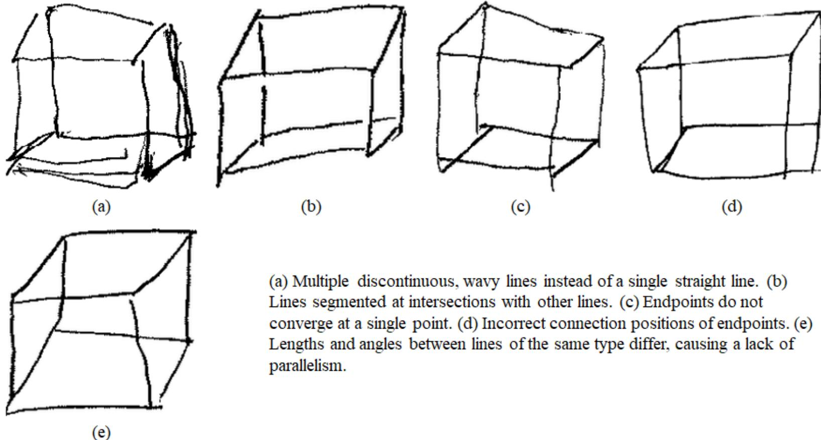
(a) Multiple discontinuous, wavy lines instead of a single straight line. (b) Lines segmented at intersections with other lines. (c) Endpoints do not converge at a single point. (d) Incorrect connection positions of endpoints. (e) Lengths and angles between lines of the same type differ, causing a lack of parallelism.
