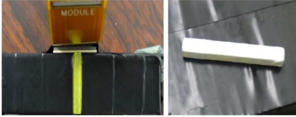
Figure 3.5 GAGG scintillator used in the experiments (Left: before shielding Right: after shielding)
