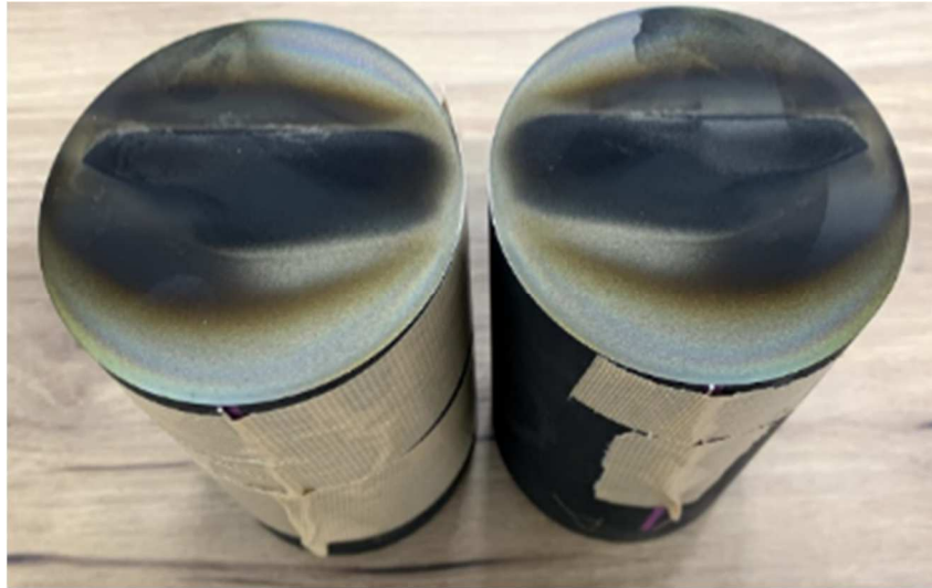
Fig. 2-9 Cutting surface with height distribution measured by ECM
