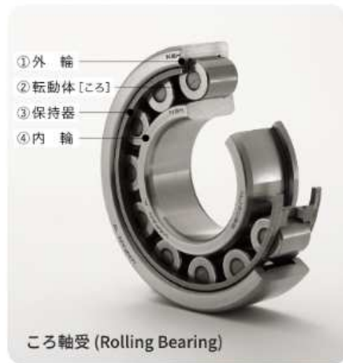
Fig. 1-1 Appearance and components of rolling bearings.
