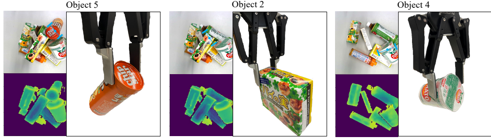
Figure 3.9: Some examples of successful grasping results in clutter scene. There are three successful cases of grasping each target object while preventing deformation and avoiding collision with other objects during grasping.
