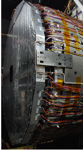
Figure 2.11: A picture of the Charged Veto detector placed in front of the CsI calorimeter.
