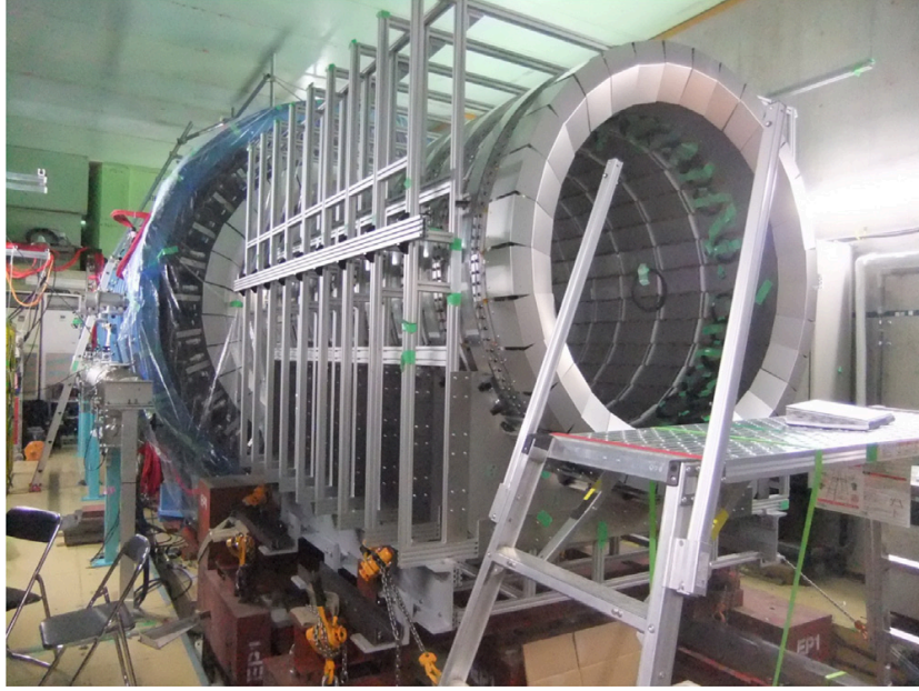
Figure 2.10: A picture of the Inner Barrel [18] during its installation, showing the arrangement of its 32 modules. The Main Barrel is also visible in the background.
