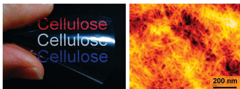
Figure 4. Digital photograph (left) and AFM image (right) of transparent TOCN film. 38
