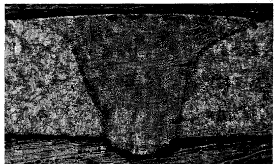
Photo. 1. An example of weld bead of AISI 304 stainless steel, 0.8 mm in thickness. Laser power=1 KW, welding speed=1 m/min.
