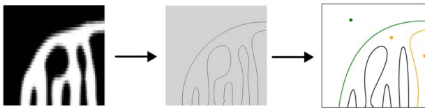
Fig. 7 Example of approximation by the Bezier curve; left: representative shape, center: contour plot, and right: approximated curve with control points
