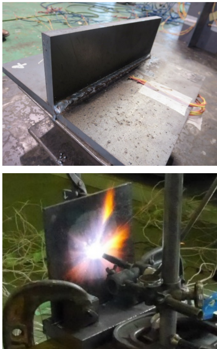
Figure 4-14 Image of the heating experiment on the T-joint specimen
