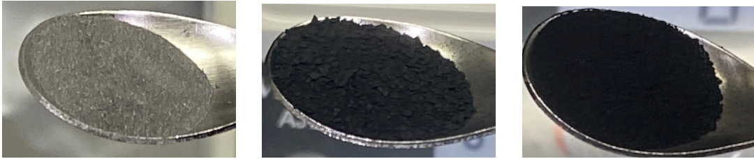
Figure 2.3: Image of sample powder: (left) Commercial vanadium nanopowder, (middle) Sample powder of S2-1 and (right) Sample powder of S2-2
