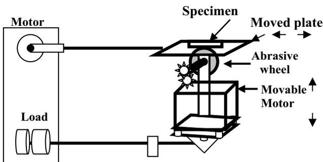
Fig. 2. Systematic diagram of abrasive wear tester.
