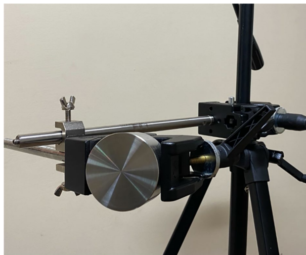
Fig. 3. Setup for transcranial static magnetic stimulation (tSMS). NdFeB magnet used for tSMS, a steel metal cylinder used for the sham.
