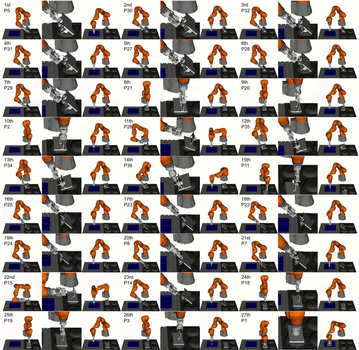
Fig. 15. The generated feasible (collision-free and IK-solvable) motions include \hat{C} , \hat{T} , and \hat{P} . The three pictures for each disassembly show the arm in a pose at the post-contact position, the zoom of the post-contact pose, and the placement pose.
