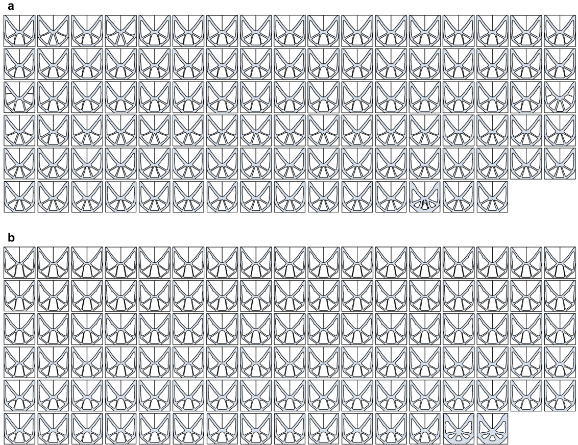
Fig. 7. Optimized designs in the two-dimensional cracked plate design problem: (a) optimized via VAE-based crossover; (b) optimized via Wasserstein crossover.
