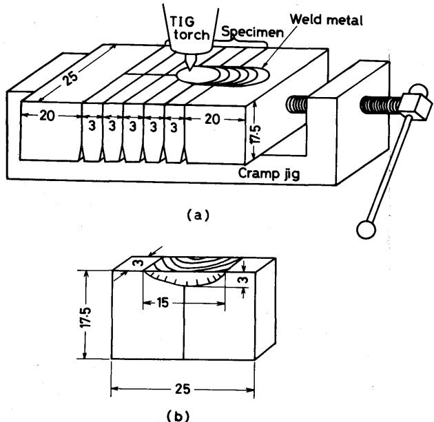
Fig. 1 Illustration of (a) welding procedure and (b) test specimen
