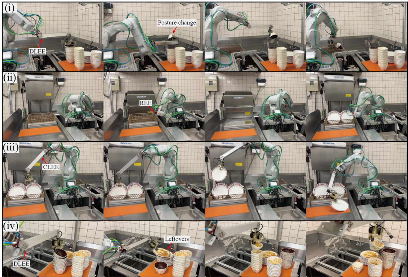
Fig. 7 Demonstration results: (i) loading used dishes onto a rack, (ii) loading the rack into the dishwasher and retrieving it after washing, (iii) unloading the washed dishes from the rack after washing, and (iv) handling dishes with leftovers
