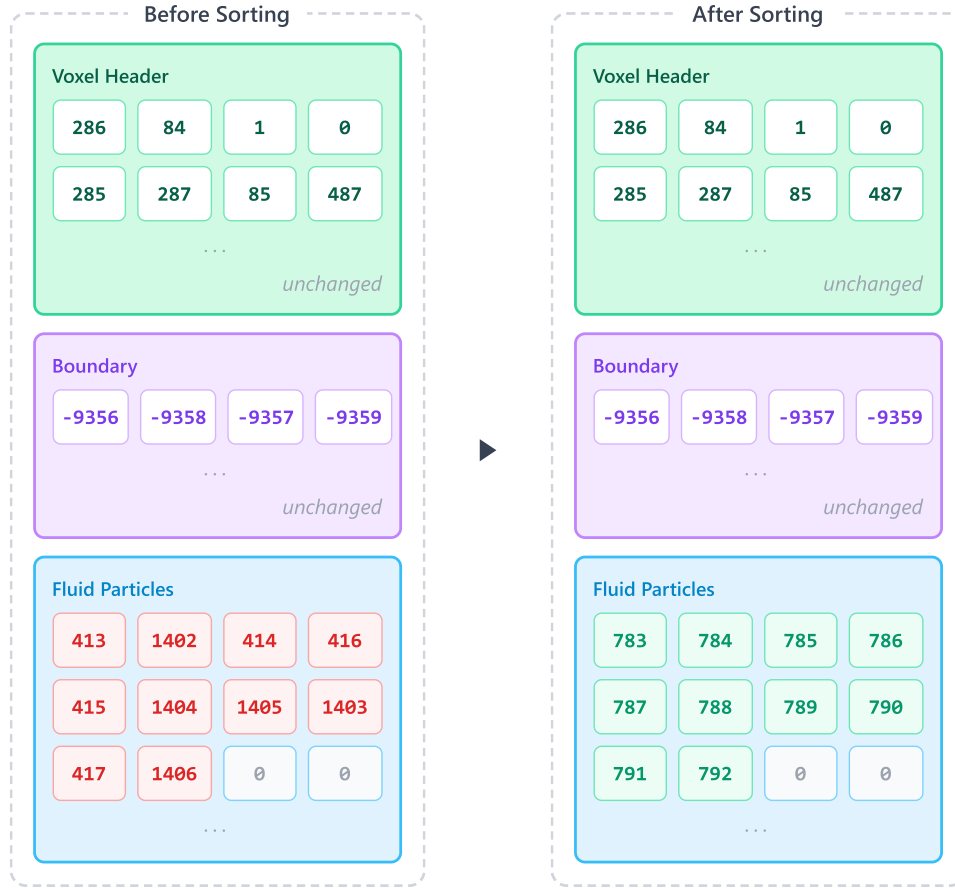
Fig. 9. One example of Cache-optimized particle resorting mechanism. The voxel structure maintains three components: spatial metadata saved in header, boundary particles with negative indices, and fluid particles. During resorting, only fluid particles are reassigned from scattered indices to contiguous sequences, while header and boundary data remain unchanged. This reorganization ensures particles within the same voxel occupy consecutive memory addresses, improving cache locality.
