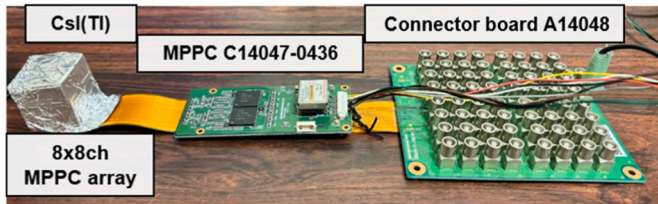
Fig. 2. Photograph of the main components of the prototype monitor CsI(Tl) scintillator (2.6 cm 3 cube), MPPC (C14047-0436, Hamamatsu photonics, Hamamatsu, Japan) and DP5 (Amptek Inc, Bedford, MA, USA).
