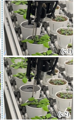
Fig. 1: (a) Arabidopsis has tiny leaves with slender petioles. They are difficult to sample. (b) Proposed system design. (c) Suction-cut sampling process: (c.1) Suction lifting the target leaf; (c.2) Cutting operation.
