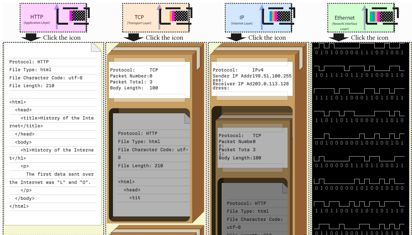
Fig. 3. In the simulator area, the contents of the data are visualized by transforming them into tangible objects, such as papers for HTTP, boxes for TCP and IP, and voltages for Ethernet.
