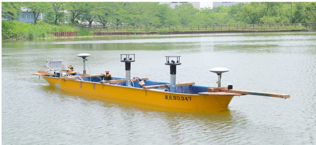
Fig. A.1: The subject ship: model-scale ship of M.V. ESSO OSAKA .
