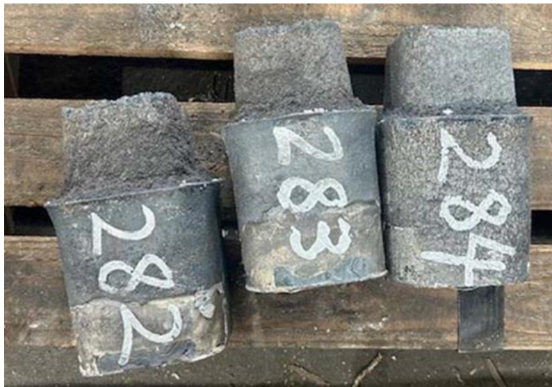
Fig. 4-1 Ingot of dummy weld metals Left: A, Center: B, Right: C.
