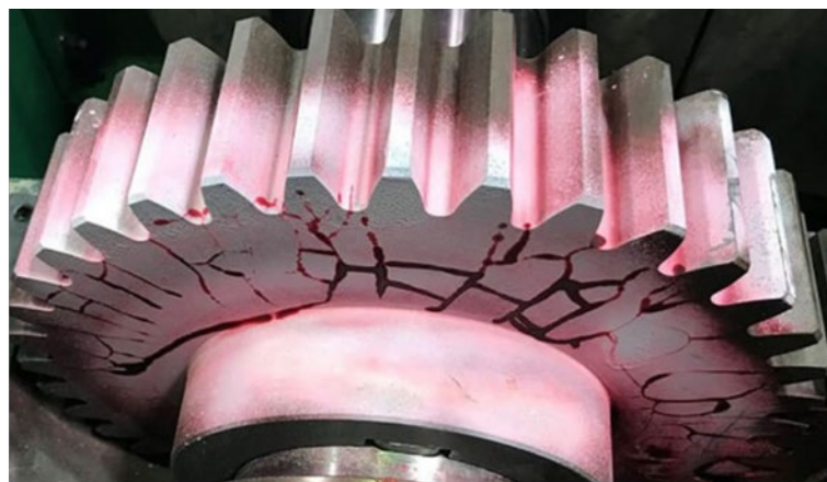
Figure 1-19 Detected cracks using penetrant testing
