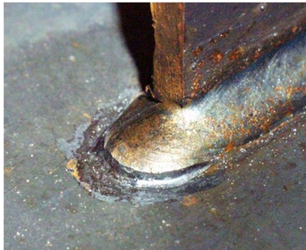
Figure 1-26 Peened weld toe [71]
