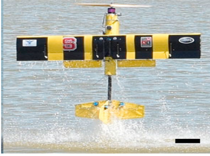
(a) EagleRay fixed-wing HAAV using fuselage-integrated ballast and drainage for transitions (Weisler et al., 2018).
