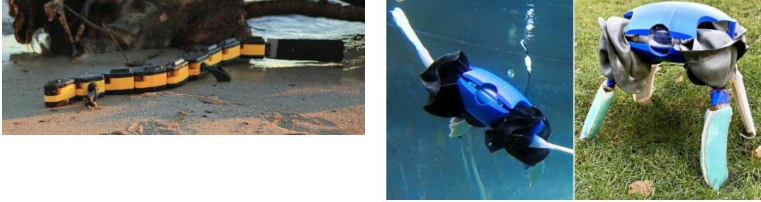
(a) AmphiBot II navigating through wetland terrain. (Crespi and Ijspeert, 2009) (b) ART (Amphibious Robotic Turtle) on land and water (Baines et al., 2022).
