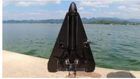
(b) Nezha SeaDart fixed-wing platform with pneumatic buoyancy and passive hydroplaning takeoff (Jin, Zeng, et al., 2025).
