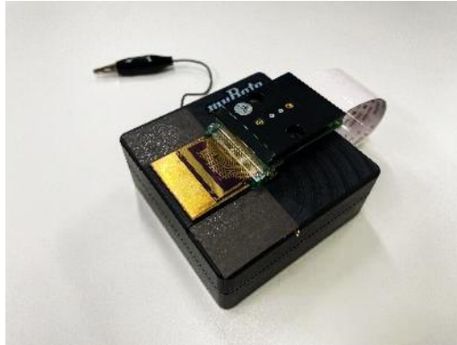
Fig 2.5. Optical image of custom-built equipment for measurement of transfer characteristics
