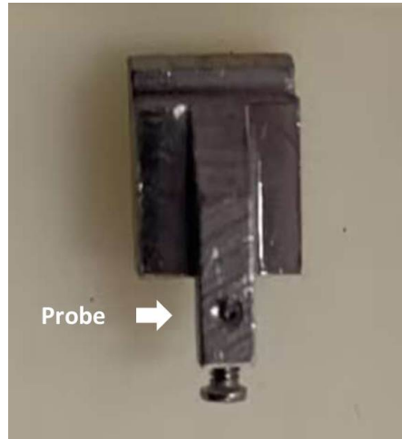
Figure 2.9: Physical image of the probe mounted on the holder.
