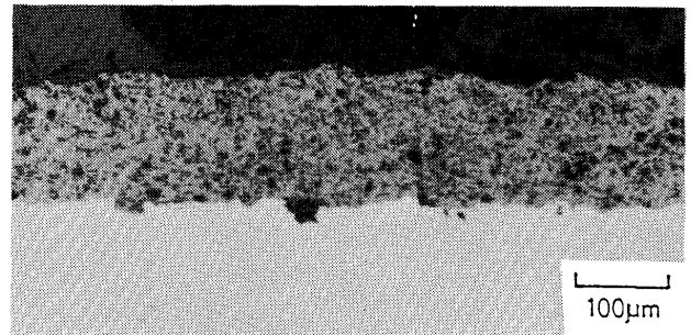
Fig. 6 Photograph of cross section of zirconia coating after heat treatment.
