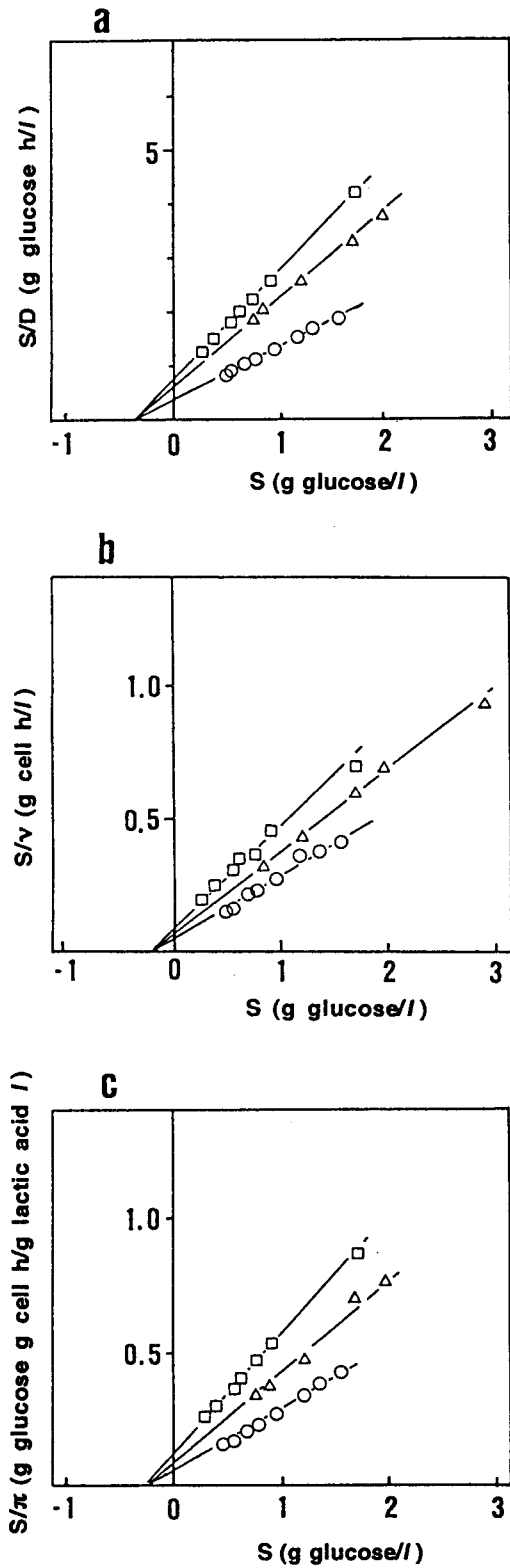
Fig. 2.3 Hofstee plots of S/D vs. S (a), S/\text{specific consumption rate of glucose } (v) vs. S (b), and S/\text{specific production rate } (\pi) vs. S (c); ○, P = 8.8 (\pm 0.5) \text{ g/l} , ( S_0 = 10 \text{ g/l} ); △, P = 16.3 (\pm 0.3) \text{ g/l} , ( S_0 = 20 \text{ g/l} ); □, P = 24.1 (\pm 1.6) \text{ g/l} , ( S_0 = 30 \text{ g/l} ).
