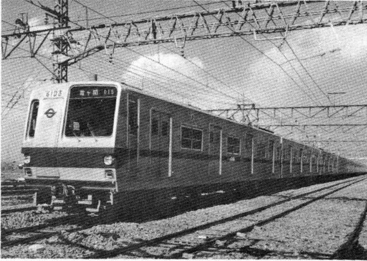
(A) Chopper controlled cars of Teito Rapid Transit Authorities in Chiyoda Line
