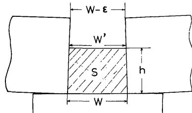
**Fig. 1** Scheme to define bead height ( $h$ ) when base metal is deformed.
