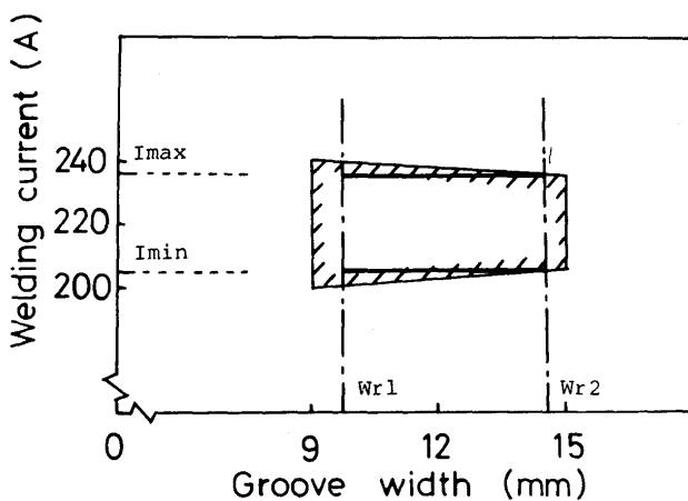
Fig. 13 Region that the cut curved surface Fig. 12(a) is projected to the plane of the welding current – groove width, in which constant current is required for control.
