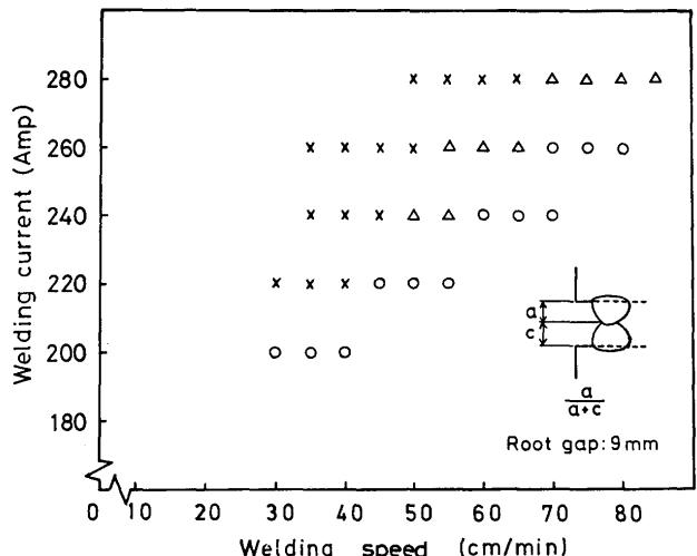
Fig. 7 Classification of bead configuration by symmetry factor.
