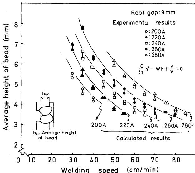
Fig. 3 Relation between bead height and welding speed for various welding currents.
