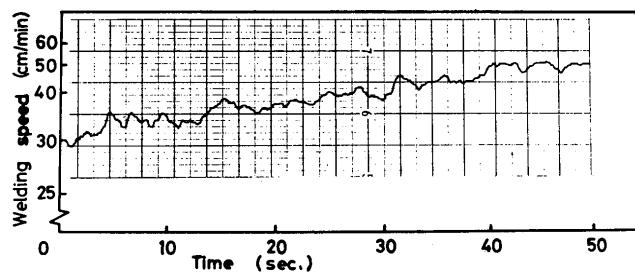
Fig. 18 Osillogram of controlled welding speed.
