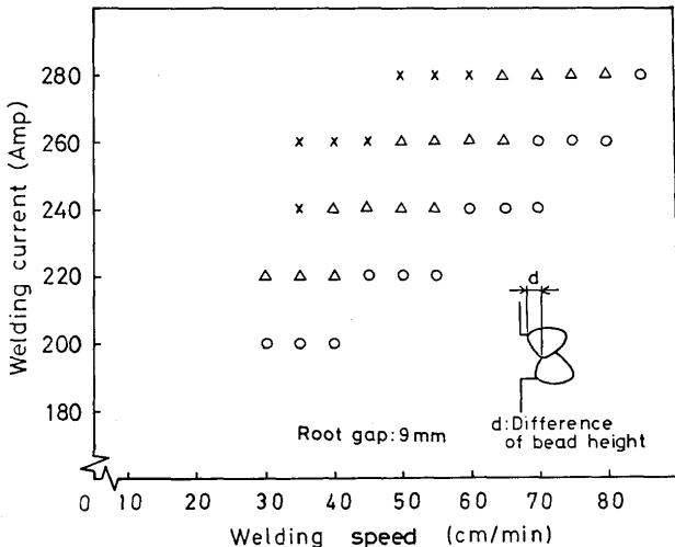
Fig. 5 Classification of bead configuration by flatness factor.
