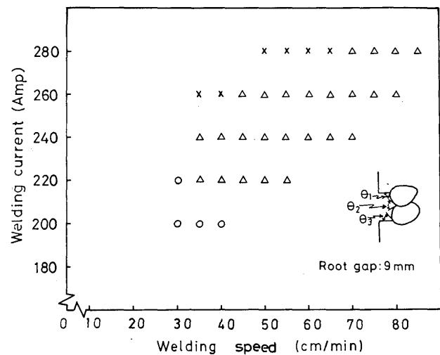
Fig. 6 Classification of bead configuration by smoothness factor.
