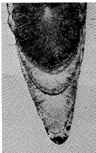
Photo. 5. Cold shut in the cross-section of SUS27 beam welds.
