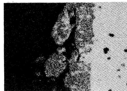
Fig. 4 SEM photograph and EDX element analysis results of cathode side interface of Cu(anode)/Zirconia/Cu(cathode) joint bonded at 1073 K for 20 min under electric field of 50 V and 1 A.
