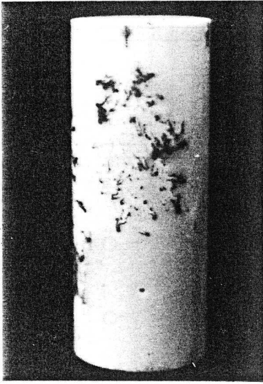
(a) FOV = 309 kV, L = 0 mm particle length = 5 mm
