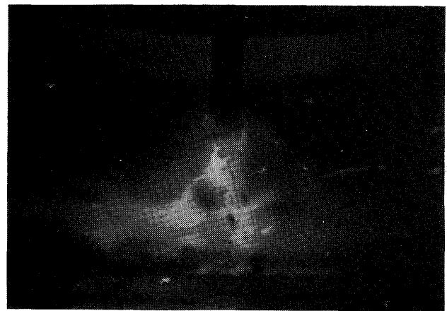
Phot. 5 Metal transfer in case of fold-shaped sheath wire.
