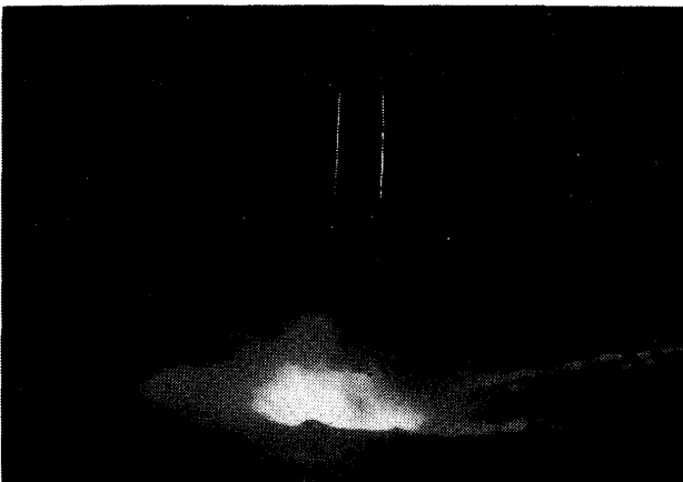
Photo. 4 Metal transfer in case of hollow-shaped sheath wire.
