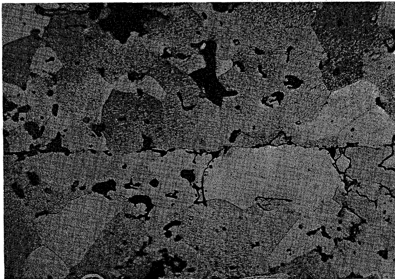
Fig. 4. Microstructure of diffusion-bonded sintered layers. Magnification 800 x, sinter FeCu, interface (W).
