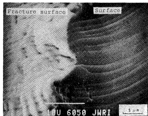
Fig. 15 Correlation between slip bands on specimen surface and feature of intergranular fracture surface in Item No. 1 (1100°C, \dot{d}_h )
