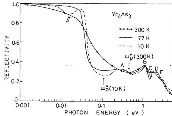
Fig. 10 Energy dependence of the optical reflectivity of Yb<sub>4</sub>As<sub>3</sub>
