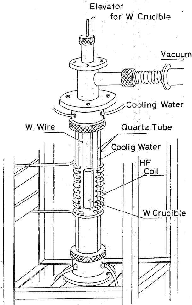
Fig. 5 Vacuum type of HF furnace in schematically
