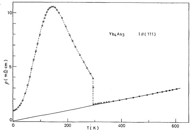
Fig. 9 Temperature dependence of the resistivity of Yb<sub>4</sub>As<sub>3</sub>
