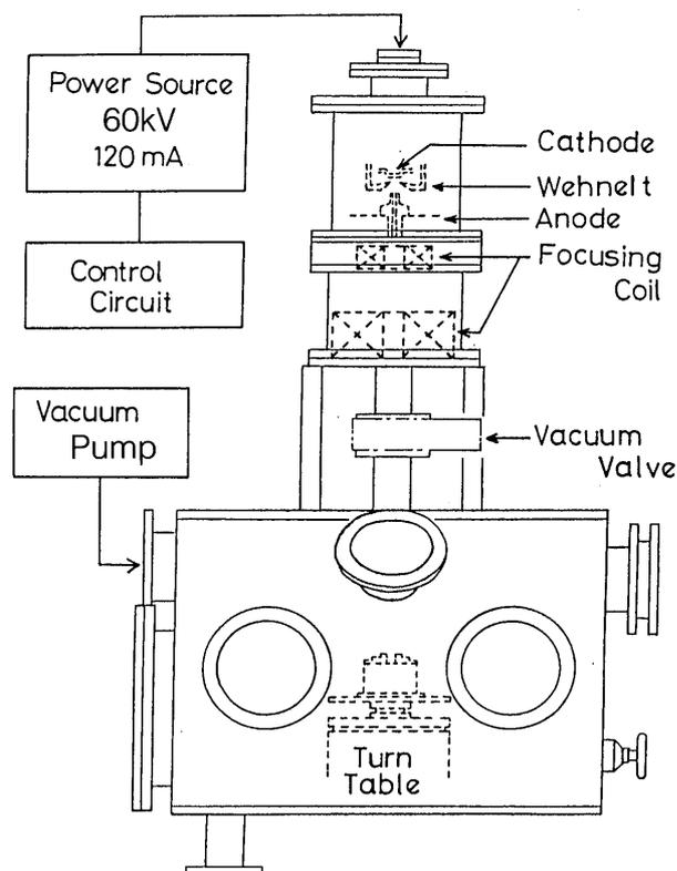
Fig. 1 Electron beam welding system for W crucible.
