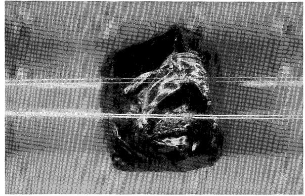
Fig. 8 Single crystal of Yb<sub>4</sub>As<sub>3</sub> obtained by new method.
