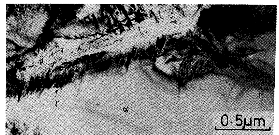
Fig. 11 Transmission electron micrographs of the specimen after charging at 4200 A/m 2 for 14.4 ks
