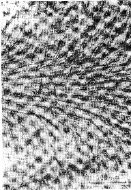
Fig. 5 Substructure-like pattern remaining at room temperature in SUS304 (120A, 15V, 130mm/min)
