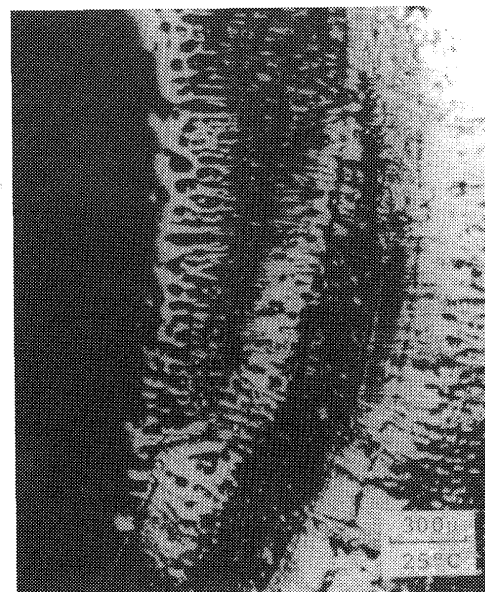
Fig. 4 Solidification front of fully austenitic stainless steel SUS310S
