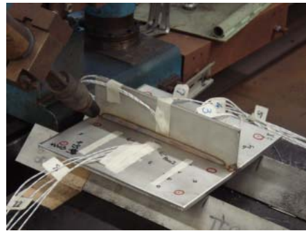
Fig.2. Experiment set up of fillet welding
