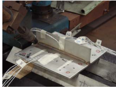
Fig.2. Experiment set up of fillet welding
