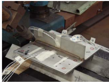
Fig.2. Experiment set up of fillet welding
