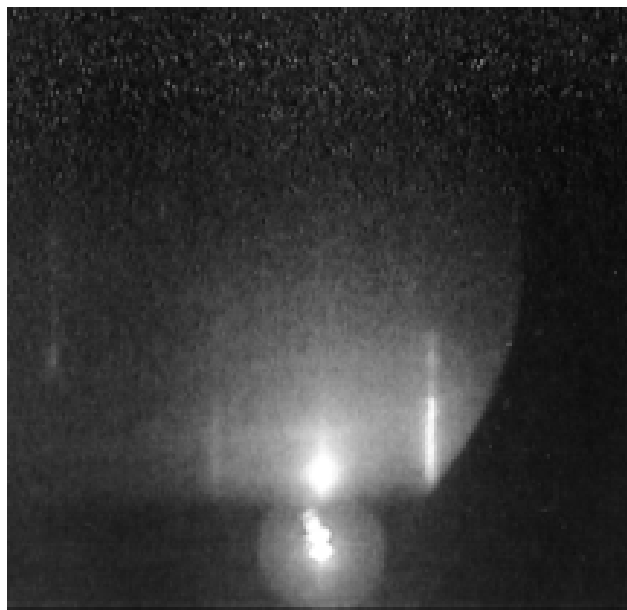
Fig. 2.6 Representative RHEED pattern of \alpha\text{-Al}_2\text{O}_3(0001) substrate. The incident direction of electron beam is \langle 1\bar{1}00 \rangle of \alpha\text{-Al}_2\text{O}_3 .
