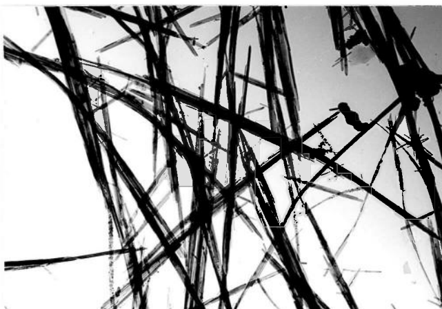
Fig. 3 Powder shape of \alpha -FeOOH seed crystal versus NaOH solution concentration varied from 0.43, 1.5, 3.5 to 7.0 mol/l under the constant concentration of \text{FeSO}_4 \cdot 7\text{H}_2\text{O} of 0.072 mol/l (Runs No. 1S ~ 4S of Table 1).
